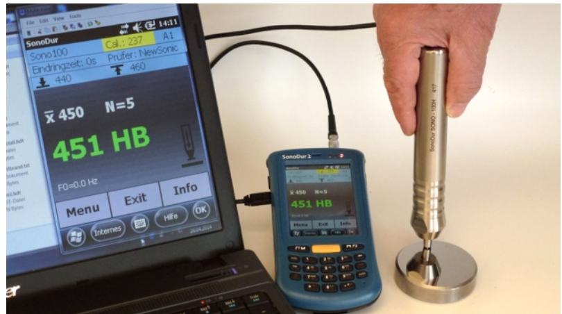
Fast and precise hardness tester the new SonoDur2 on GGG50 cast iron and remote control via PC
